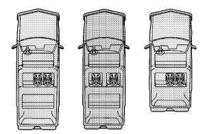
Your vehicle has the LATCH system. You will find anchors (A) in the center and right side passenger second row seating positions for bench seats and the outboard passenger positions for bucket seats. This system, designed to make installation of child restraints easier, does not use the vehicle's safety belts. Instead, it uses vehicle anchors (A, B) and child restraint attachements to secure the restraints. Some restraints also use another vehicle anchor to secure a top tether strap (C).
